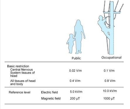
For exposures of the general public, the ICNIRP reference levels for 50 Hz magnetic and electric fields are 200  $\mu$ T and 5 kV/m respectively. These limits apply to both children and adults. Since the established effects of interest, as described in Factsheet 5, are instantaneous, the purpose of controls is to limit maximum exposure at any point in time. As such there is no greater effect associated with long term exposures than with short term exposures.
